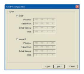
If the DHCP server is unavailable or not found, the user will be prompted to configure the TCP/IP settings of the Print Server manually by clicking "Yes" on the screen below. Clicking "No" will make the Print Server search for the IP address from a DHCP server on the network.
